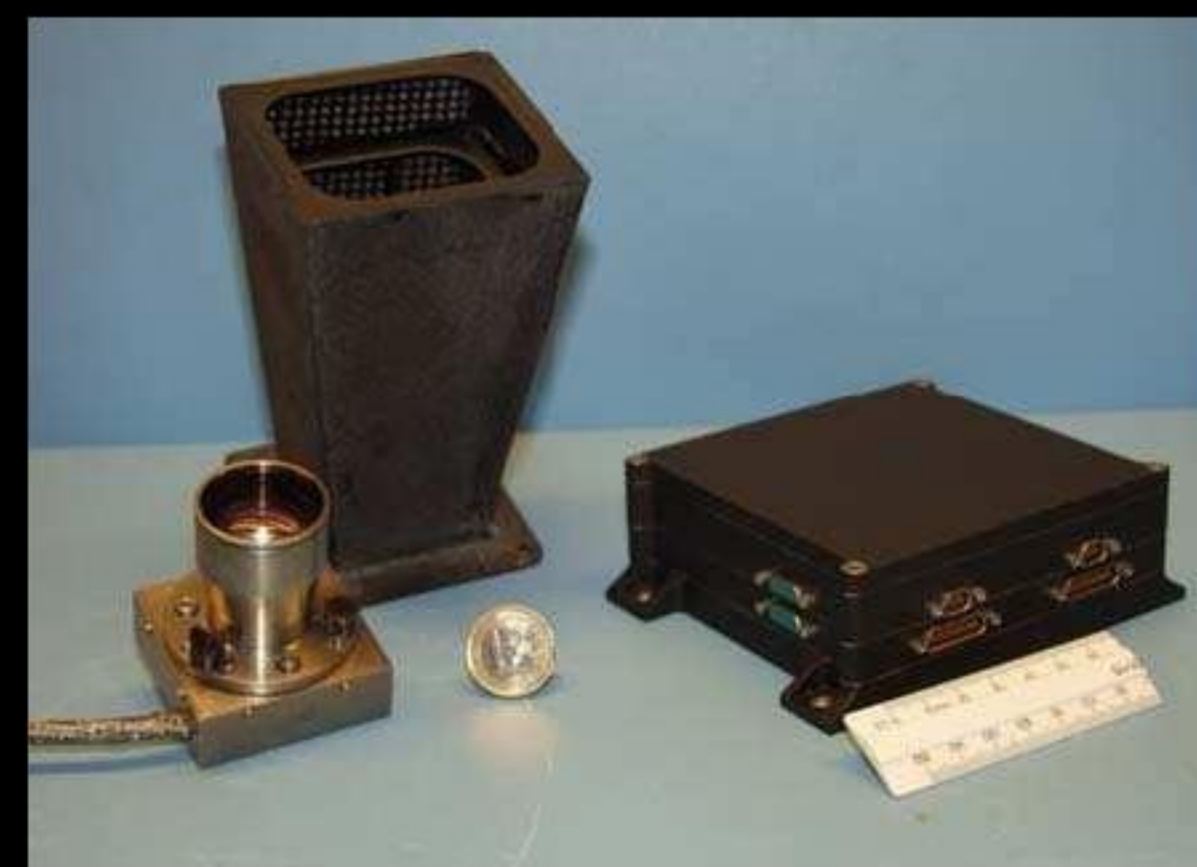
Pictured above are the Denmark Technical University (DTU) star trackers.
