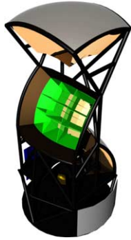
Fig. 1. The “reference design” of EXIST, with three Tungsten coded-mask imaging telescopes ( 2.7 \text{ m}^2 of CZT per telescope).
