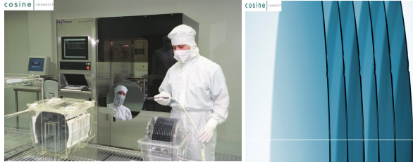
Wafer dicing and ribbing (1 mm pitch, 0.2 mm width)
