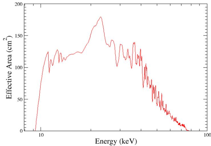
**Figure 4 Effective area for HXI. No significant difference is present for the two mirror area curves used for the response generation.**
