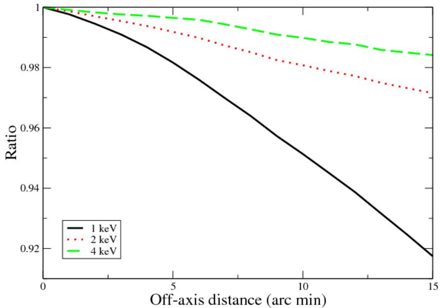
**Figure 5 The ratio of vignetting for a reduced outer radius compared to the radius for which the vignetting curves were calculated at 1, 2, and 4 keV**
