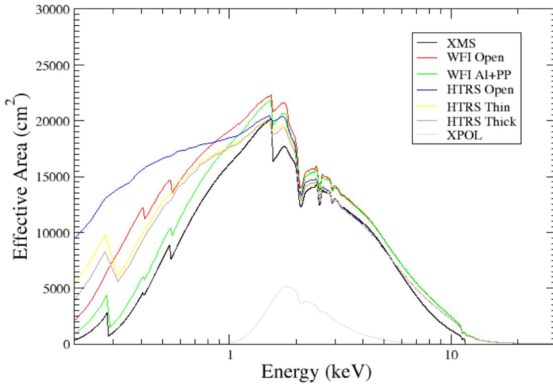
**Figure 3 Instrumental effective areas for the 2.5m<sup>2</sup> minimum design**
