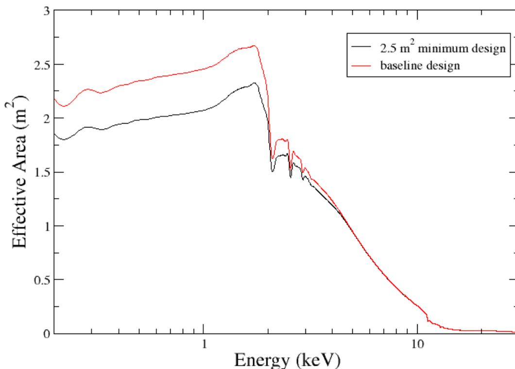
**Figure 1 Mirror effective area, including obscuration by the gratings and loss factors, as function of energy for the baseline design and the 2.5 m<sup>2</sup> mirror effective area (see text).**
