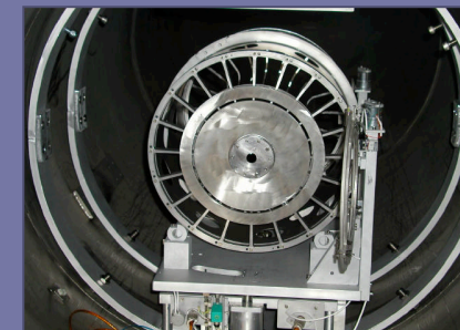
2 nested nickel mirror shells in X-ray test at PANTER
