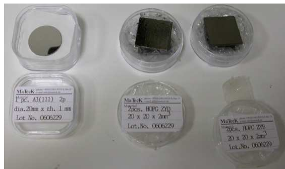
Fig. 6. From left to right: aluminum and graphite crystals built by Matek. Graphite crystals differ from the amplitude of domains misalignment.
